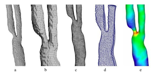
Figure 2: Meshing stages: (a) binary image, (b) initial mesh, (c) surface mesh after cosmetics, (d) a cut off view of the volumetric mesh. (e): time-averaged WSS distribution.
